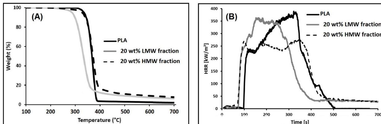
Figure 6 : TGA curves (under nitrogen, 20 °C/min) and HRR curves (35 kW/m<sup>2</sup>) of PLA containing LMW and HMW lignin fractions. Adapted from <sup>19</sup>.
