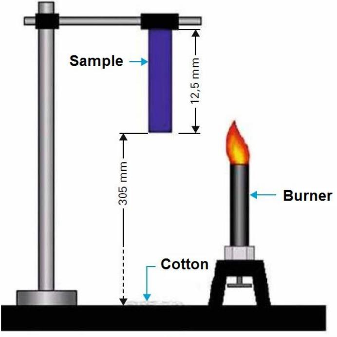
Figure 2: Schematic representation of vertical UL94 test.
