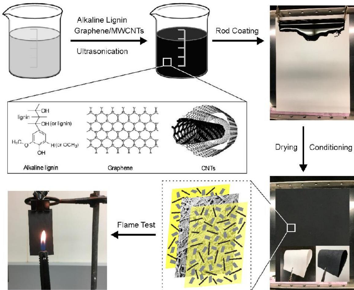
Figure 8 : Schematic presentation of the fabrication process and fire test of the paper coated with lignin, carbon nanotubes and graphene combination. Reproduced from <sup>27</sup> with permission.
