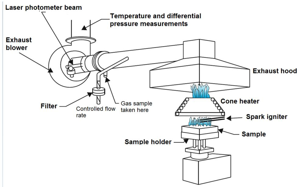
Figure 1: Schematic representation of cone calorimeter apparatus. Different parts of the apparatus are named and specified.
