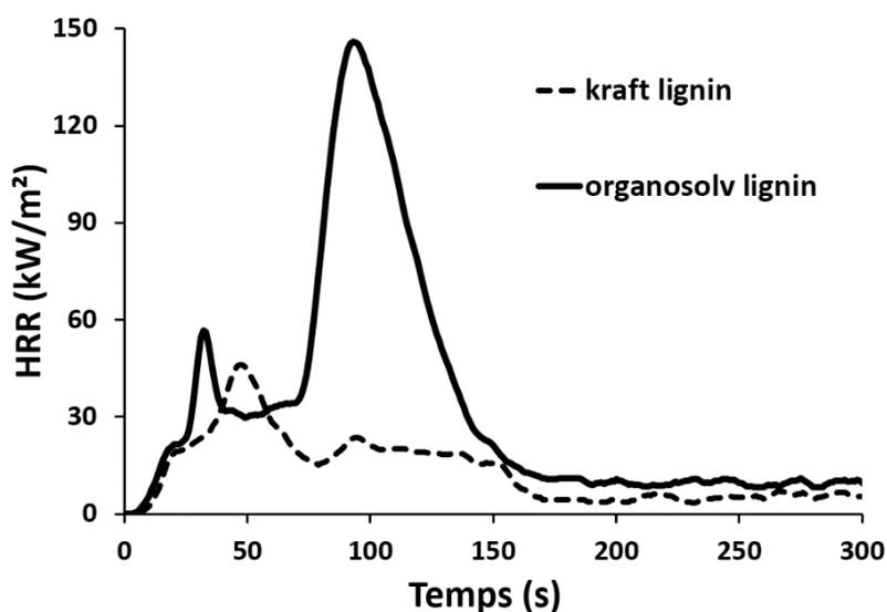
Figure 3 : Heat release rate (HRR) curves obtained from cone calorimeter test of kraft lignin and organosolv lignin (35 kW/m<sup>2</sup>). Reproduced from<sup>13</sup> with permission.
